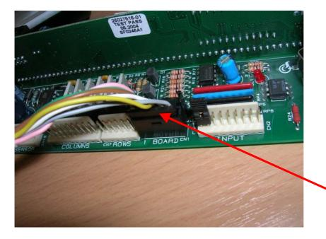
The jumper is on the first and second pin. This is the position of the vega /BVM snack **B**
